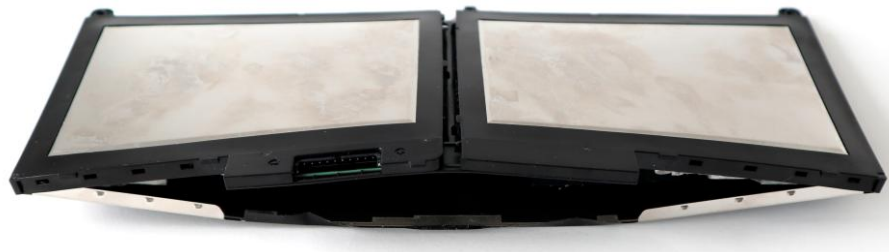
Laptop battery pressurized by thermal runaway
